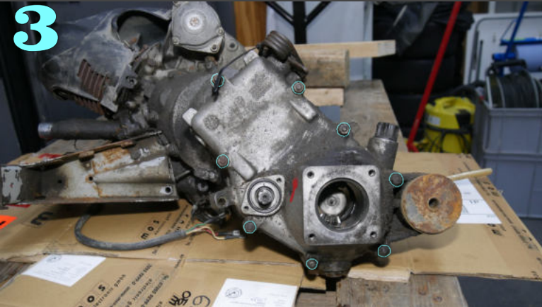
Unscrew the marked screws and remove the casing
