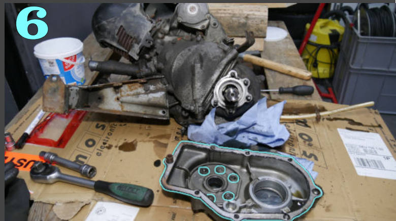
Remove the rest of the casing
