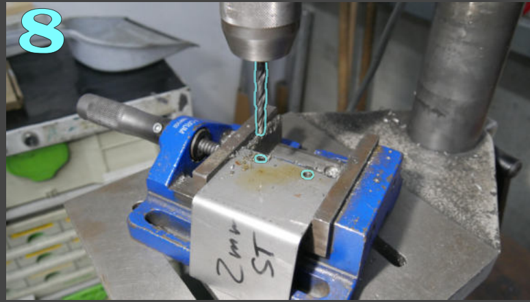
Holes for roof bolting
