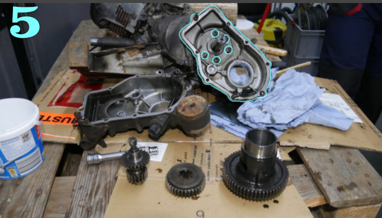
Unscrew the screws located inside the casing
